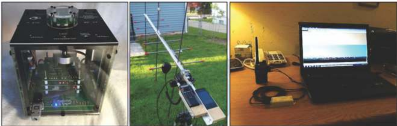
Figure 1 - (a) EyaSat Classroom Satellite Kit, (b) Ham Radio Communication, (c) Packet Radio Communication
